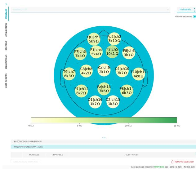
**Figure 16.** Interface widget for real-time impedance visualizer. OpenBCI EEG cap for 16 channels is used within our MI paradigm.
