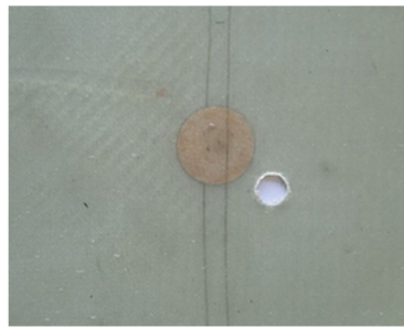
Figure 3. Smart PMC plate with a 10 mm diameter hole.
