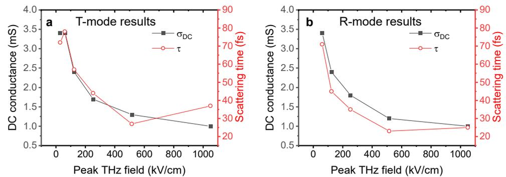
**Figure 4.** (a) DC conductance and scattering time obtained from Drude fits at various incident peak THz field strengths from the transmission-mode THz-TDS measurements. Solid squares: DC conductance. Open circles: scattering time. (b) The same parameters extracted from Drude fits reflection-mode measurements.
