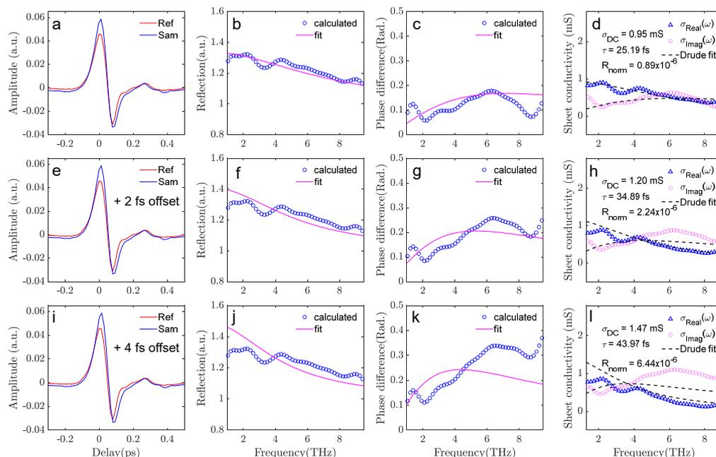
**Figure 5.** Phase offset correction of the reflection-mode THz-TDS data analysis. (a–d) With optimum offset correction, the extracted conductance spectra match the best with the Drude model. The calculated reflection and phase difference curves also match best with the fit. (e–h) With 2 fs extra phase offset, the extracted parameters show significant deviation from the Drude model fits. (i–l) With 4 fs extra offset, a Drude fit is impossible in the broad frequency range.
