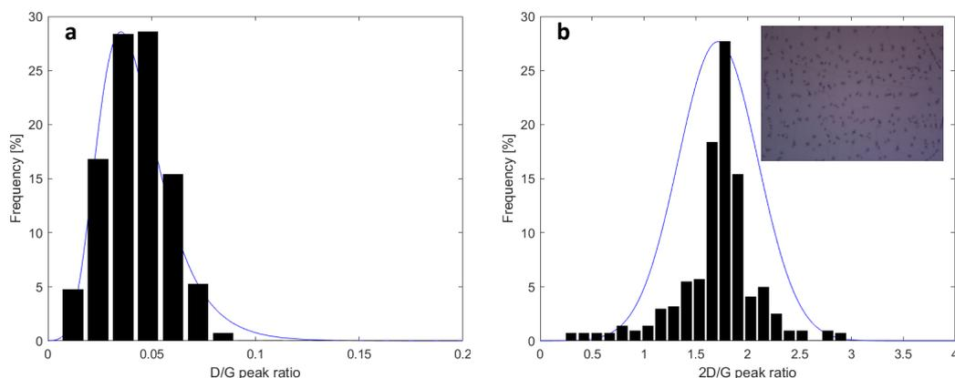
**Figure 2.** (a) The Raman histogram of the ratio of D band to G band intensity. (b) The Raman histogram of the ratio of the 2D band to G band intensity. Inset, an optical image of the graphene.
