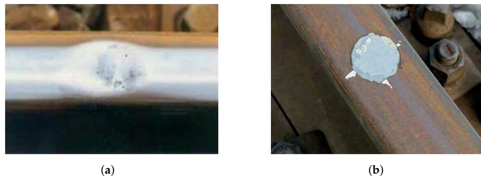
Figure 3. A real and an artificial squat: (a) A real squat. (b) An artificial squat in the testbed.
