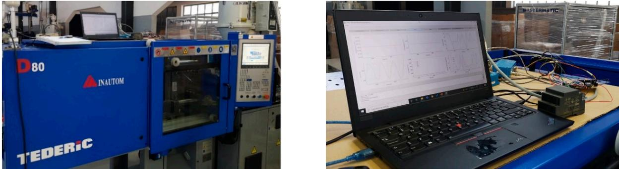
**Figure 9.** Test setup with the working monitoring system and injection molding machine.
