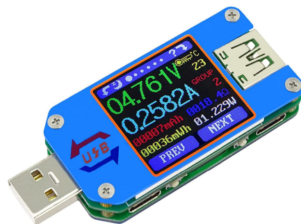
Figure 6. USB power meter tester used to estimate the power consumption.
