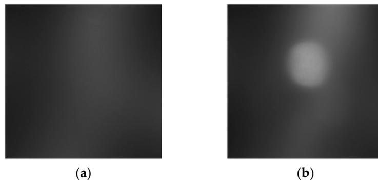
Figure 29. Tactile-sensation images by size: (a) 8 mm, (b) 12 mm.
