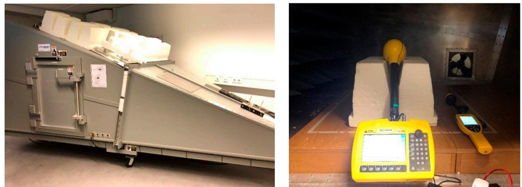
**Figure 2.** GTEM cell outside and inside. Benchmark equipment (SRM3006) inserted in the GTEM cell.
