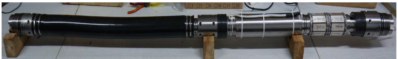
Figure 4. Internal actual picture of an acoustic sonde composed of an azimuthal-transmitting arc array.
