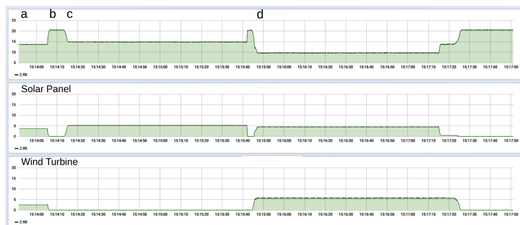
Figure 13. Power distribution with two intermittent power sources, collected from AC grid hardware modules and visualized with Grafana. Initially (time point a), both renewable sources are active and the transformer (i.e., the larger utility grid) supplies only the difference. When one or both renewable sources fail (b, c), the transformer power output rises to compensate for the shortfall, but returns to lower levels when renewable energy is again supplied (d).
