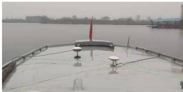
**Figure 21.** Installation position of GNSS antenna.
