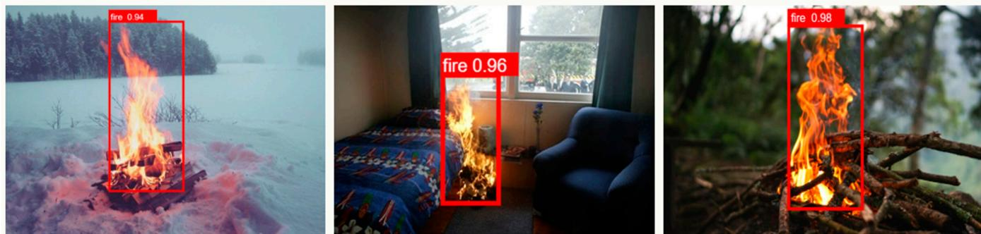
**Figure 8.** Results of fire detection system for day images.
