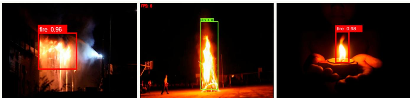
**Figure 9.** Results of fire detection system for night images.
