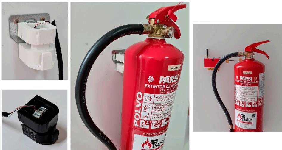
Figure 7. Powder hook design and complete system assembled.
