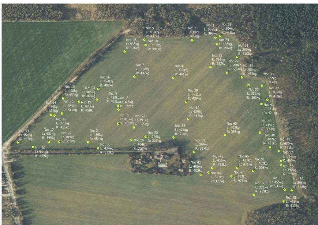
Figure 15. An example of a bale distribution map, with information on maximum compaction.
