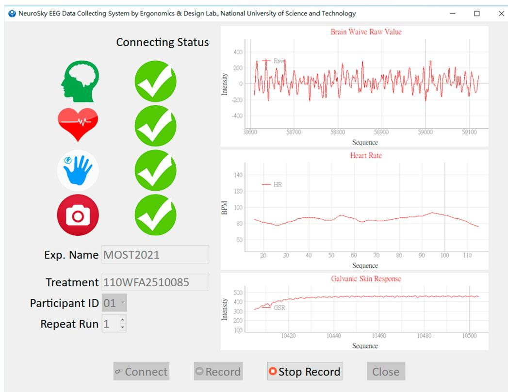
**Figure 4.** GUI of the low-cost biofeedback platform developed in this study.
