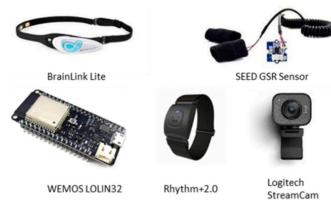
**Figure 3.** The biometrical sensor, devices, and development board used in this study. The total cost of these devices was about USD 800, which is a significant cost saving when compared with a medical-grade system.
