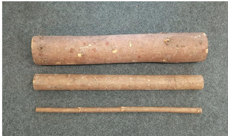
**Figure 7.** Logs of different diameters used in the grasping experiments. Big log (top) has a diameter of 13.5 cm, medium log (middle) has a diameter of 7.5 cm and small log (bottom) has a diameter of 2.5 cm.
