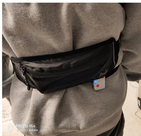
**Figure 5.** The attached IMU to the participant’s shimmer for data collection during straight walking.
