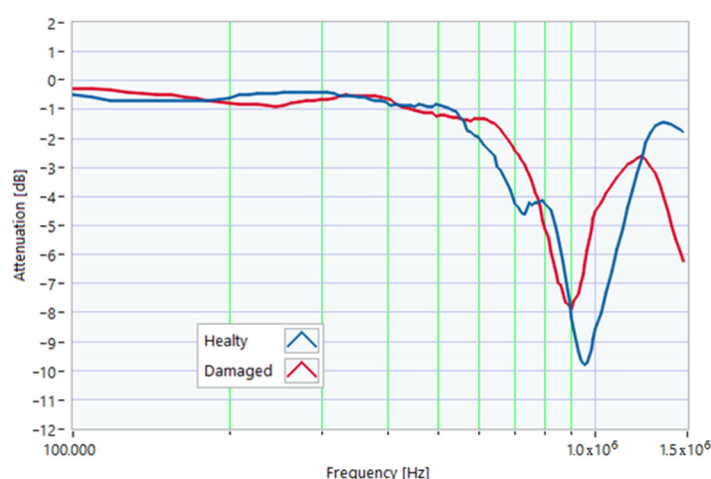
Figure 18. Comparison between TFs of the same motor in healthy conditions and after overheating.
