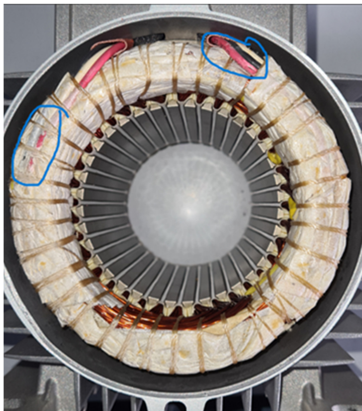
Figure 20. The stator of an induction motor after a fall from a height of 1 m.
