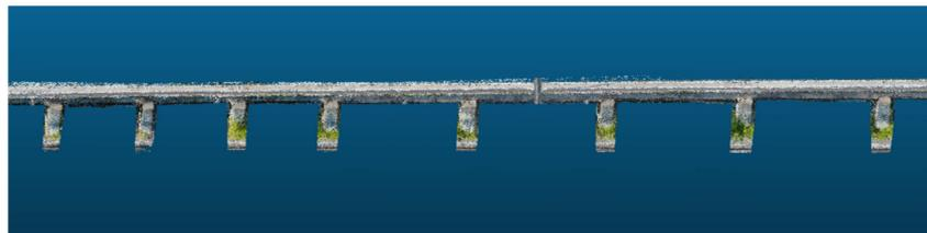
**Figure 14.** Illustration of the dense point clouds of the magnetic floating linear structure.
