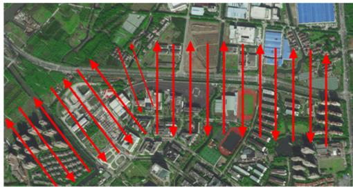
**Figure 7.** Oblique photography route plan of the magnetic levitation test line.
