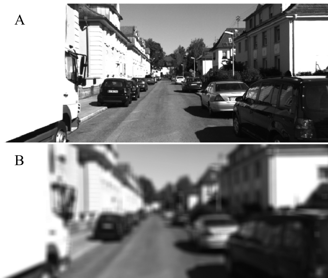
Figure 2. Sample image from the original (A) and blurred (B) KITTI dataset (sequence 07). The original image was blurred using a gaussian filter with a patch size of 12 pixels and a standard deviation of 2.15 pixels 241 in both directions.
