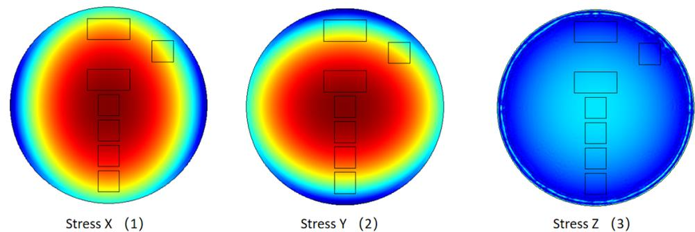
**Figure 9.** The internal stress field of the PVDF layer in the three directions computed by the FE model.
