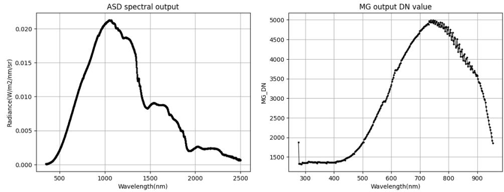
Figure 9. ASD spectral radiance and photodetector spectral response curve under the same light conditions.
