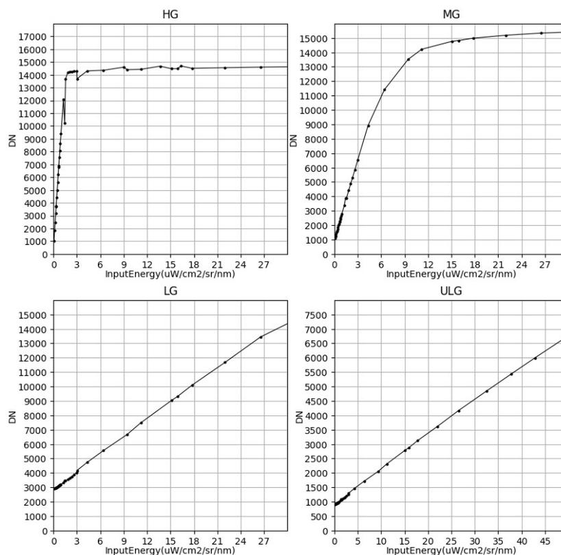
Figure 11. Four gains’ response curve.
