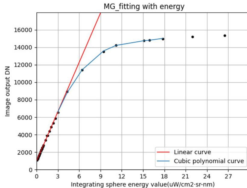
**Figure 12.** Fitting curve of the laboratory absolute radiometric response of MG.
