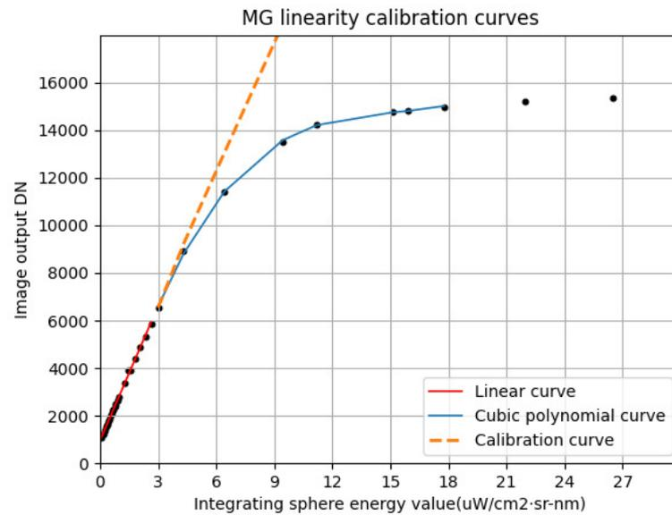
Figure 13. Response curve after nonlinear correction.
