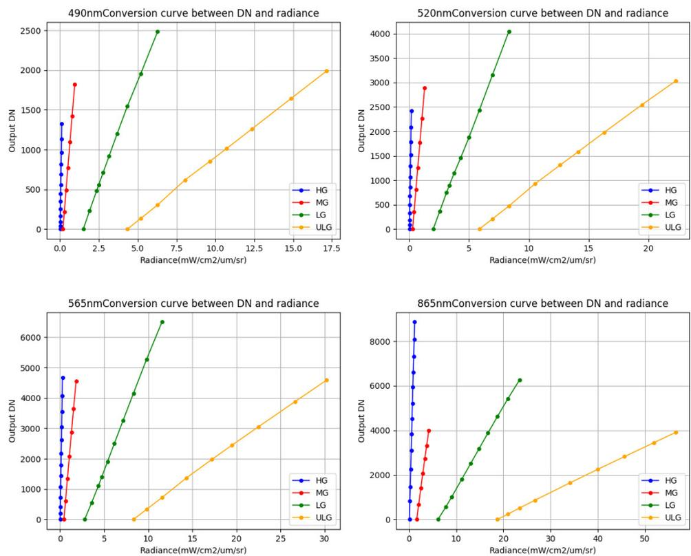
Figure 10. Photodetector response curves of four spectral channels with the radiance detected with ASD as reference.
