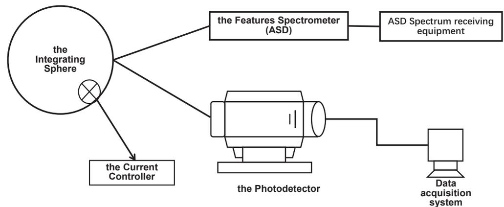
**Figure 5.** Experimental design diagram for the determination of the absolute radiometric calibration coefficient.
