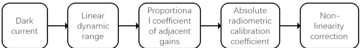
**Figure 3.** Flowchart of the laboratory calibration of an adaptive-gain imaging system.
