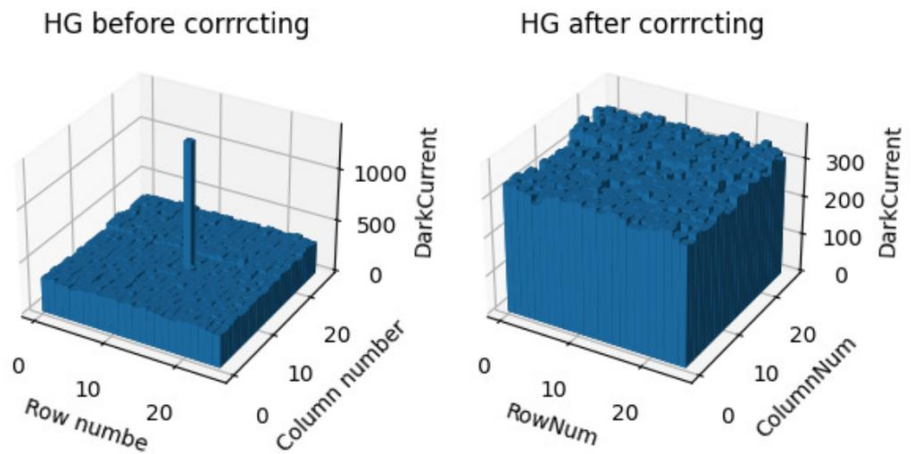
**Figure 6.** Comparison before and after bad-pixel correction.
