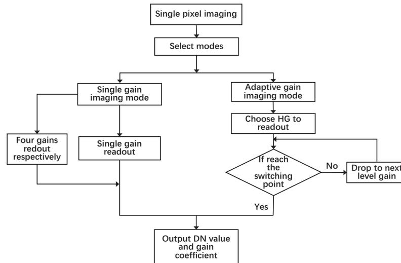
**Figure 1.** Flowchart of single-pixel imaging mode.
