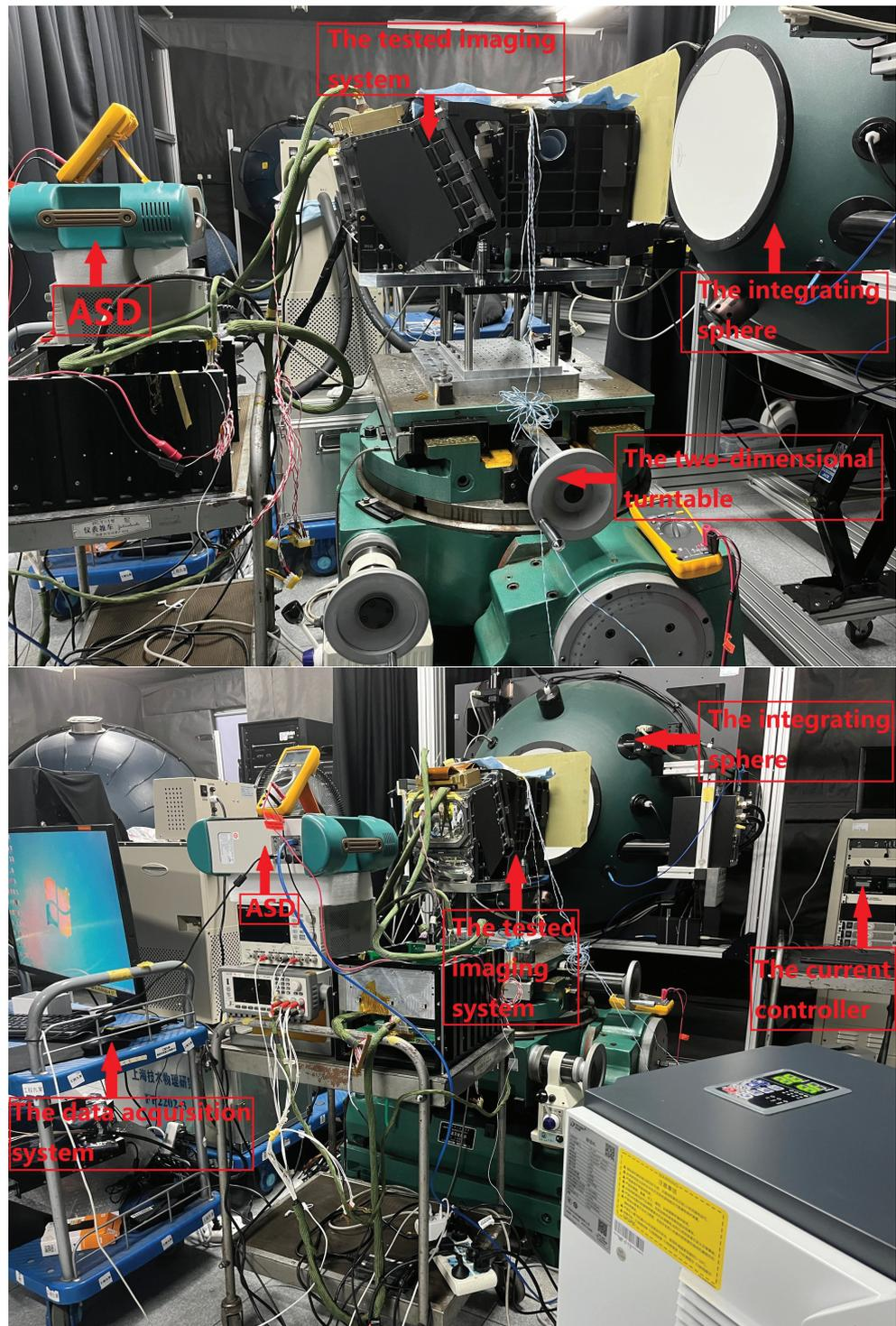
Figure 4. Laboratory radiation calibration system.
