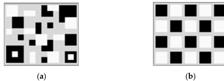
Figure 2. SSVEP stimulus pattern (size: 3 cm × 4 cm). (a) QR code pattern; (b) Checkerboard pattern.
