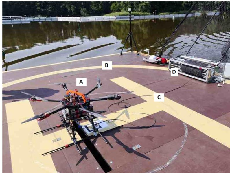
**Figure 3.** Mutlirotor UAV (A), landing pad (B), power cord (C) and automatic winch (D).
