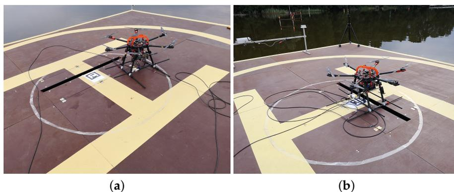
**Figure 18.** Tethered multicopter landing: (a) worst result—landing at a distance of 61 cm from the center of the landing pad; (b) best result—landing at a distance of 31 cm from the center of the landing pad.
