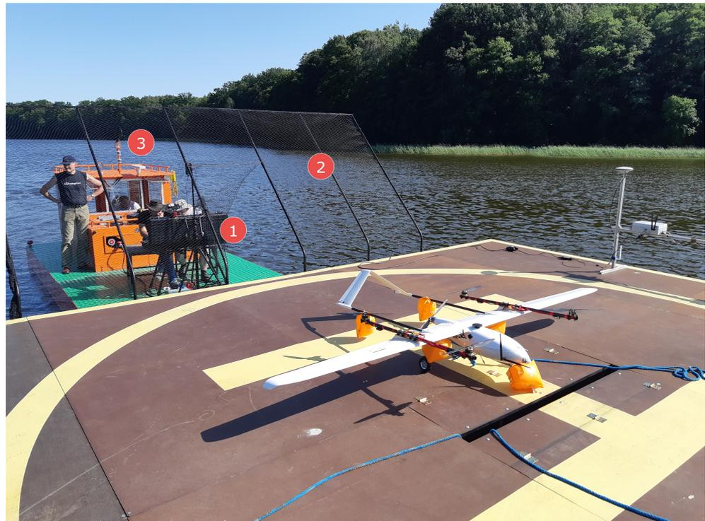
**Figure 6.** Albatross VTOL and floating landing pad view, 1—UAVs' ground control station, 2—a safety net, 3—a push barge.
