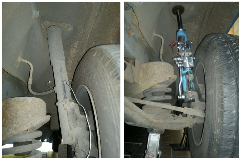
Figure 18. On the left factory damper and on the right PZD-FT damper built into the suspension of a commercial van vehicle.
