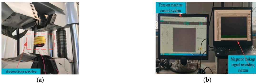
**Figure 16.** X70 steel strip tensile test device. (a) Tensile testing machine. (b) Software control systems and signal acquisition systems.
