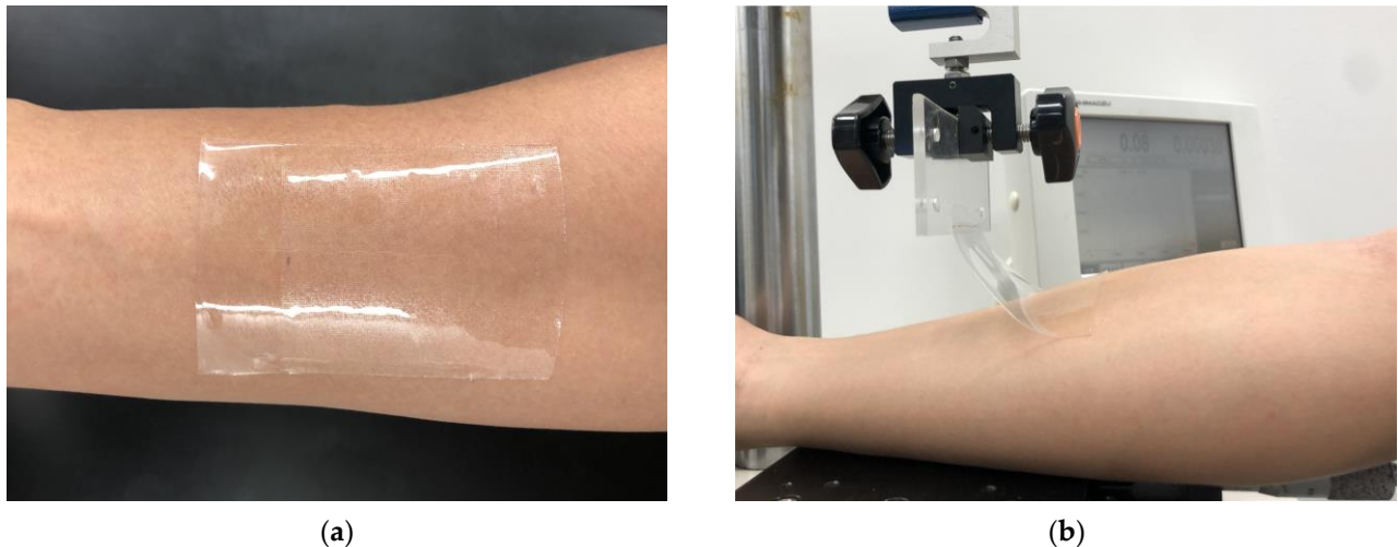
Figure 5. Peel tests for sensor. (a) Pasting point; (b) Photo of peel test.
