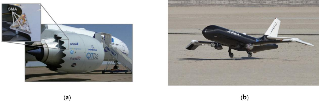
**Figure 5.** Examples of SMA materials in the aviation industry: (a) SMA-based shape control at Boeing 777-300ER airplane engines [78]; (b) SMA torque tubes are mounted in the chord-wise direction along the hinge-line to control the articulation of the outboard wing section.
