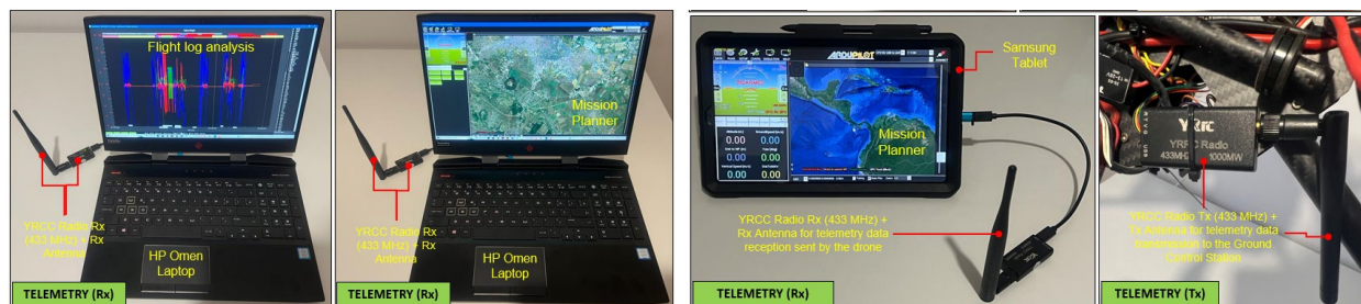
Figure 7. Arrangement of the telemetry kit on the drone and on the ground.
