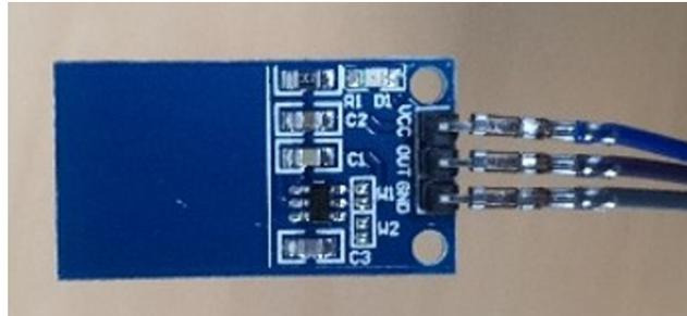
**Figure 1.** A capacitive sensor.
