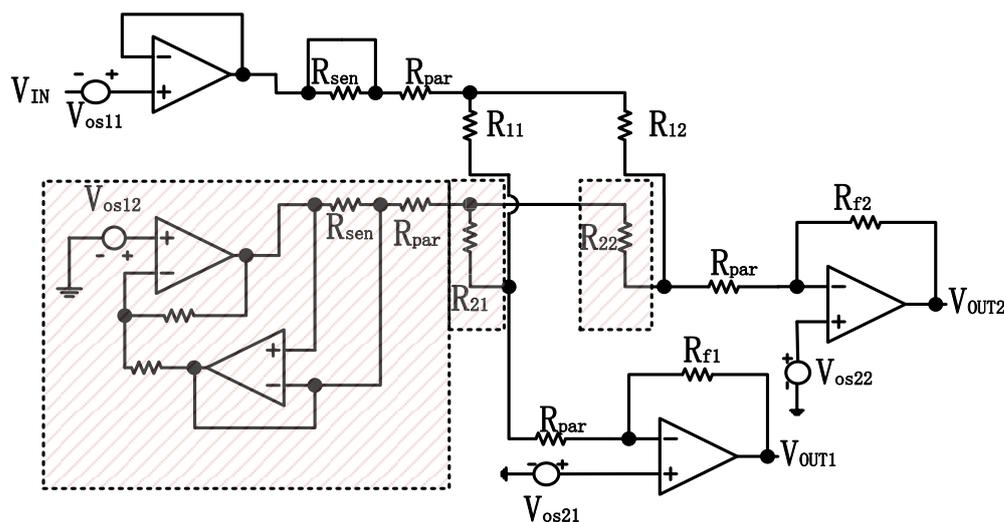
**Figure 5.** A  $2 \times 2$  array circuit model including parasitic effects and crosstalk current effect for DZCM.
