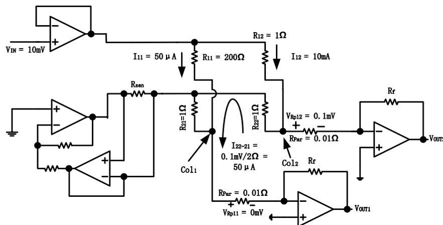
Figure 8. Simplified  $2 \times 2$  array circuit example to demonstrate singular values effect in DZCM.
