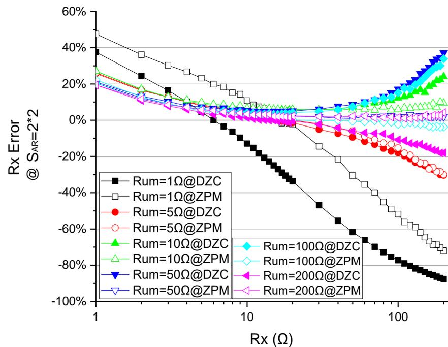
**Figure 9.** The effect of  $R_x$  on measurement error of different  $R_{um}$  when  $S_{AR} = 2 \times 2$  in DZCM and ZPM (EXP B).
