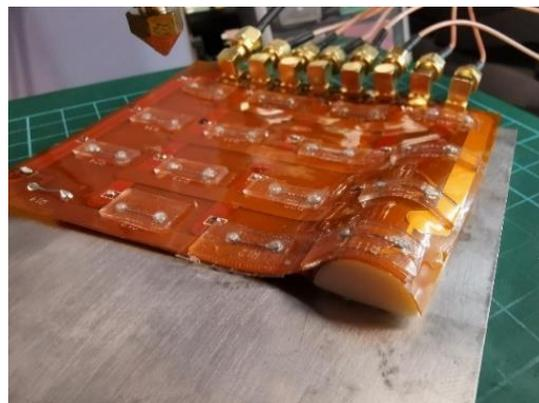
**Figure 14.** Flexible sensor mounted onto bending surface with thumb-like size.
