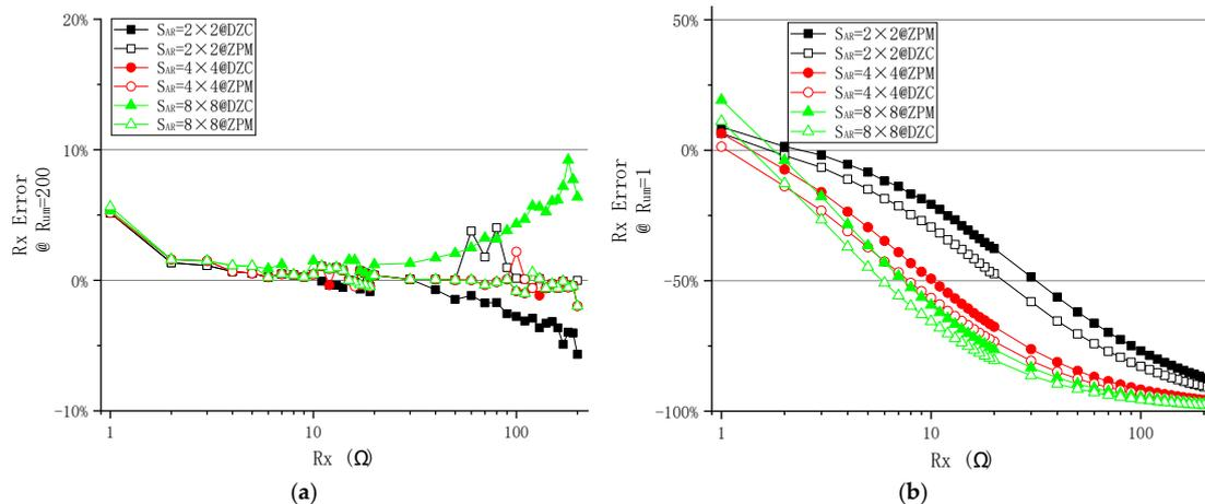
Figure 7. The effect of  $R_x$  on measurement error of different  $S_{AR}$  when (a)  $R_{um} = 200 \Omega$  and (b)  $R_{um} = 1 \Omega$  in DZCM and ZPM (EXP A).
