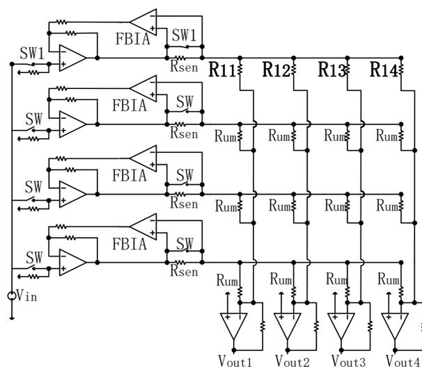
Figure 3. The circuit design of DZCM for a 4 × 4 array.
