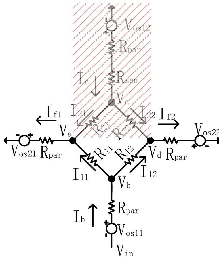
**Figure 6.** DZCM array network extracted and analyzed with Kirchhoff's law.
