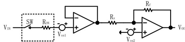
**Figure A2.** Circuit designs that include parasitic effects in the cases of ZPM.
