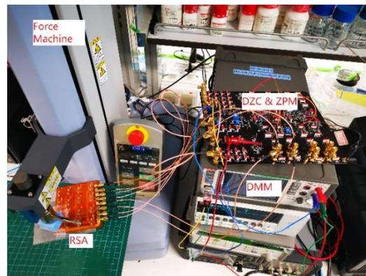
**Figure 13.** Force sensor test bench.
