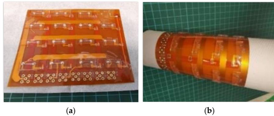
**Figure 12.** EGeIn based  $4 \times 4$  flexible RSA (a) on flat surface and (b) on bending surface.
