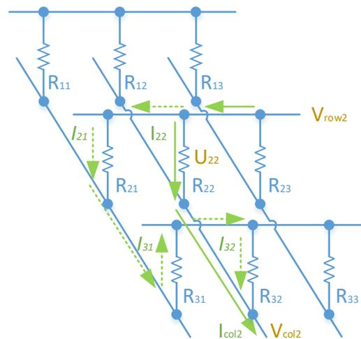
**Figure 1.** Crosstalk currents induced in the resistor array.
