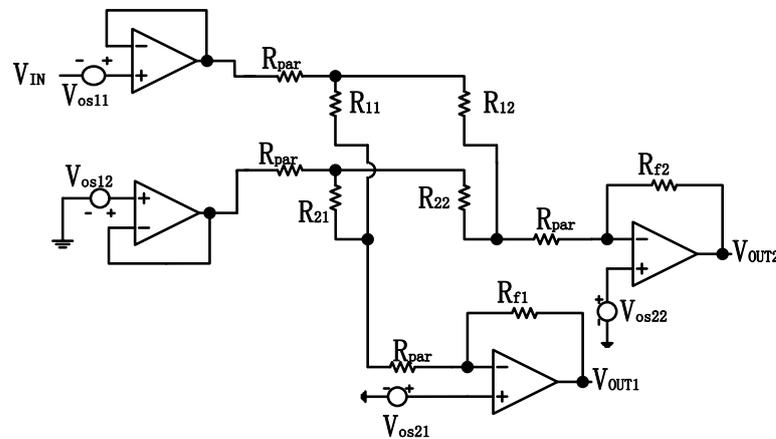
**Figure A3.** A  $2 \times 2$  array circuit model including parasitic and crosstalk current effects for ZPM.
