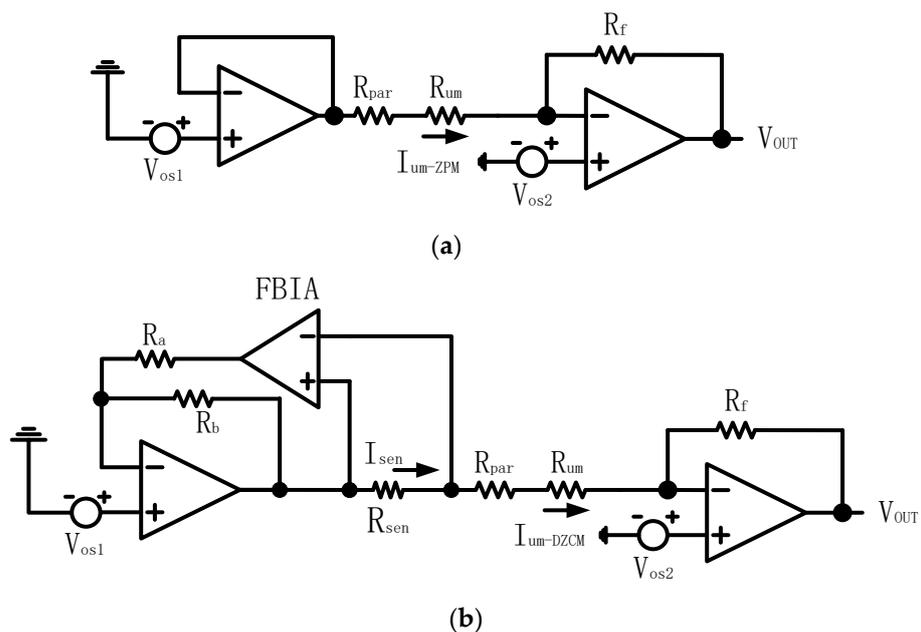
Figure 4. Simplification network with one unmeasured resistor of (a) ZPM and (b) DZCM.
