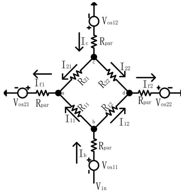
**Figure A4.** Array network extracted and analyzed with Kirchhoff's law.
