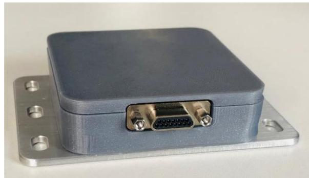
Figure 3. SpW-to-UWB WIU hardware.
