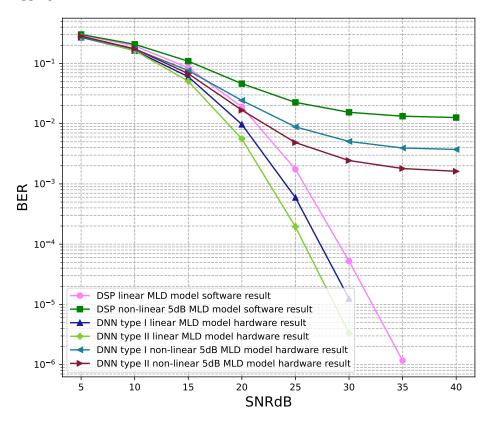
**Figure 24.** BER versus SNR for the receiver hardware architectures with M = 4, MLD is used and the clipping level of the nonlinear PAs is 5 dB.
