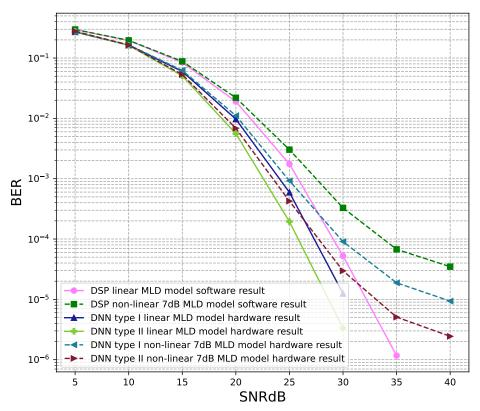
**Figure 25.** BER versus SNR for the receiver hardware architectures with M = 4, MLD is used and the clipping level of the nonlinear PAs is 7 dB.
