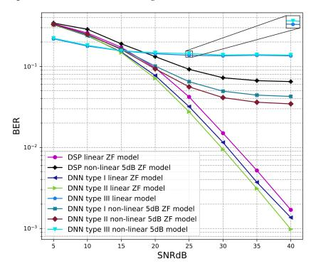
**Figure 16.** BER versus SNR for the proposed receivers with M = 4, ZF is used and the clipping level of the nonlinear PAs is 5 dB.
