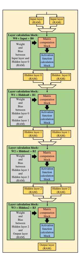
Figure 6. General neural network hardware architecture.
