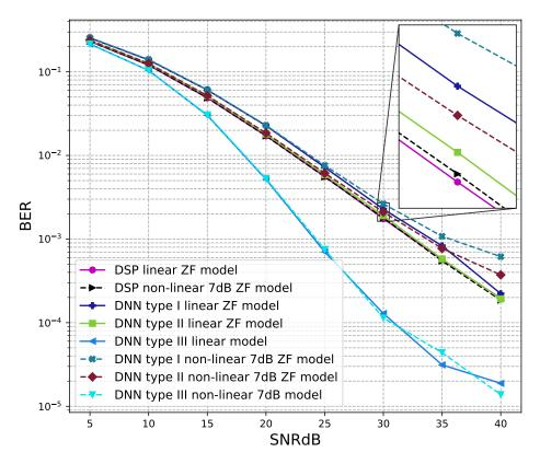
**Figure 14.** BER versus SNR for the proposed receivers with M = 2, ZF is used and the clipping level of the nonlinear PAs is 7 dB.
