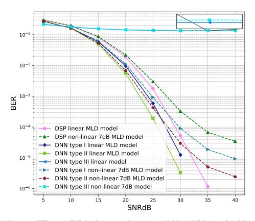
**Figure 19.** BER versus SNR for the proposed receivers with M = 4, MLD is used and the clipping level of the nonlinear PAs is 7 dB.
