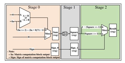
Figure 10. The simplified Sigmoid hardware design.
