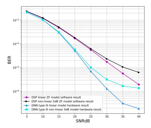
**Figure 20.** BER versus SNR for the receiver hardware architectures with M = 2, ZF is used and the clipping level of the nonlinear PAs is 5 dB.
