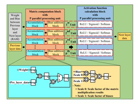
Figure 11. Layer data calculation block with quantization technique.
