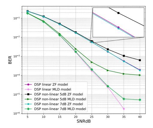
Figure 12. BER versus SNR for the conventional receivers with M = 2.
