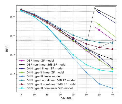
**Figure 13.** BER versus SNR for the proposed receivers with M = 2, ZF is used and the clipping level of the nonlinear PAs is 5 dB.
