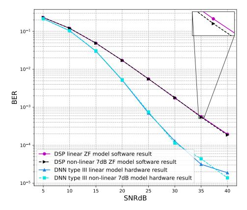
**Figure 21.** BER versus SNR for the receiver hardware architectures with M = 2, ZF is used and the clipping level of the nonlinear PAs is 7 dB.
