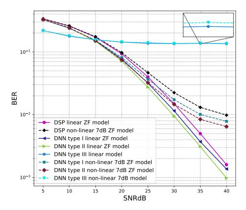
**Figure 17.** BER versus SNR for the proposed receivers with M = 4, ZF is used and the clipping level of the nonlinear PAs is 7 dB.
