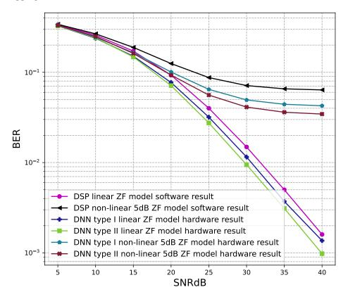
**Figure 22.** BER versus SNR for the receiver hardware architectures with M = 4, ZF is used and the clipping level of the nonlinear PAs is 5 dB.
