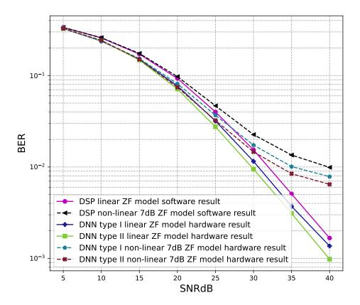
**Figure 23.** BER versus SNR for the receiver hardware architectures with M = 4, ZF is used and the clipping level of the nonlinear PAs is 7 dB.
