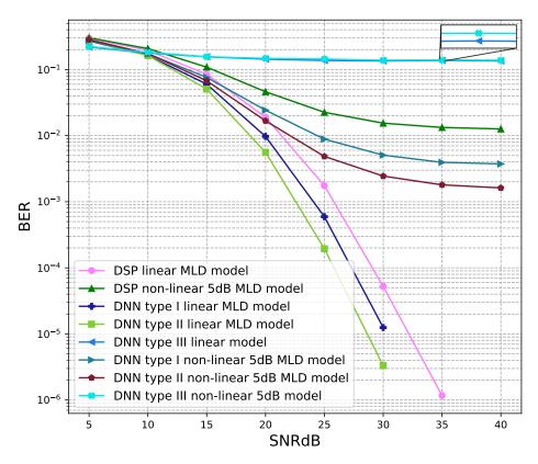
**Figure 18.** BER versus SNR for the proposed receivers with M = 4, MLD is used and the clipping level of the nonlinear PAs is 5 dB.
