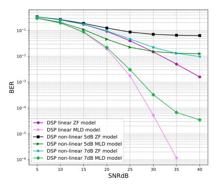
Figure 15. BER versus SNR for the original receivers with M = 4.
