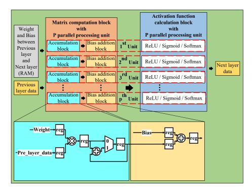
Figure 7. Layer data calculation block.
