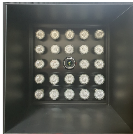
Figure 5. Halogen lamp device of 5 \times 5 array type. Infrared camera placed in the center.
