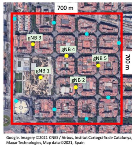
**Figure 3.** Map included in the scenario topology model of the implemented RAN NDT. The positions of the considered gNBs correspond to the yellow dots on the map.
