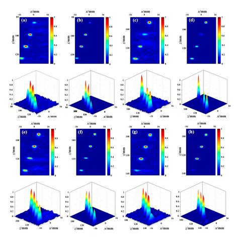
**Figure 6.** The PCSV and (PCSV)  $\sigma$  factors of different defects covered by the interface echo: PCSV and its 3D display of (a) the fourth defect covered; (c) the fifth defect covered; (e) the sixth defect covered; (g) the seventh defect covered; and PCSV with  $\sigma = 2$  and its 3D display of (b) the fourth defect covered; (d) the fifth defect covered; (f) the sixth defect covered; (h) the seventh defect covered.
