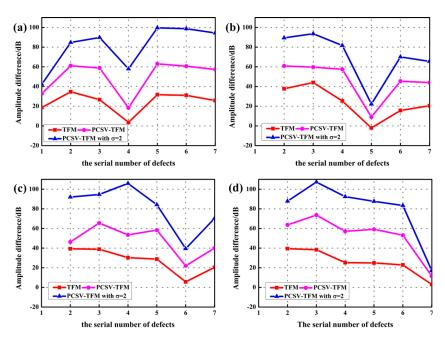
**Figure 9.** The amplitude difference between defects and the undesired echo around them at the depth of (a) the fourth defect covered; (b) the fifth defect covered; (c) the sixth defect covered; (d) the seventh defect covered; by using TFM, PCSV-TFM, and PCSV-TFM with power exponent  $\sigma = 2$ .
