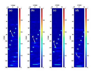
**Figure 5.** The PCSV factor images of different defects covered by the interface second echo: (a) the fourth defect covered; (b) the fifth defect covered; (c) the sixth defect covered; (d) the seventh defect covered.
