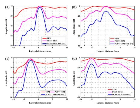
**Figure 8.** The lateral variations at the depth of (a) the fourth defect covered; (b) the fifth defect covered; (c) the sixth defect covered; (d) the seventh defect covered; by using TFM, PCSV-TFM, and PCSV-TFM with power exponent  $\sigma = 2$ .
