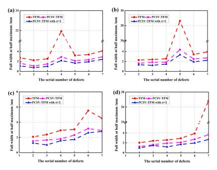
**Figure 10.** The full width at half maximum at the depth of (a) the fourth defect covered; (b) the fifth defect covered; (c) the sixth defect covered; (d) the seventh defect covered; by using TFM, PCSV-TFM, and PCSV-TFM with power exponent  $\sigma = 2$ .
