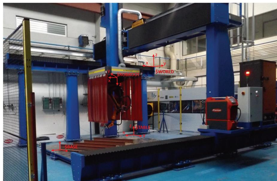
Figure 9. A super flexible shipbuilding welding robot unit with 9 degrees of freedom [128]. Reprinted with permission from [128].
