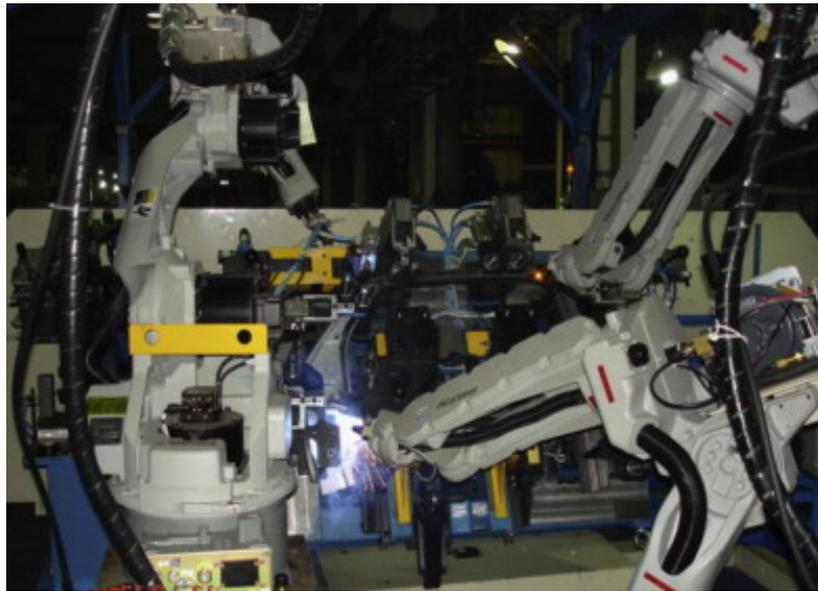
**Figure 10.** Welding robot for automobile door production [133]. Reprinted with permission from [133].
