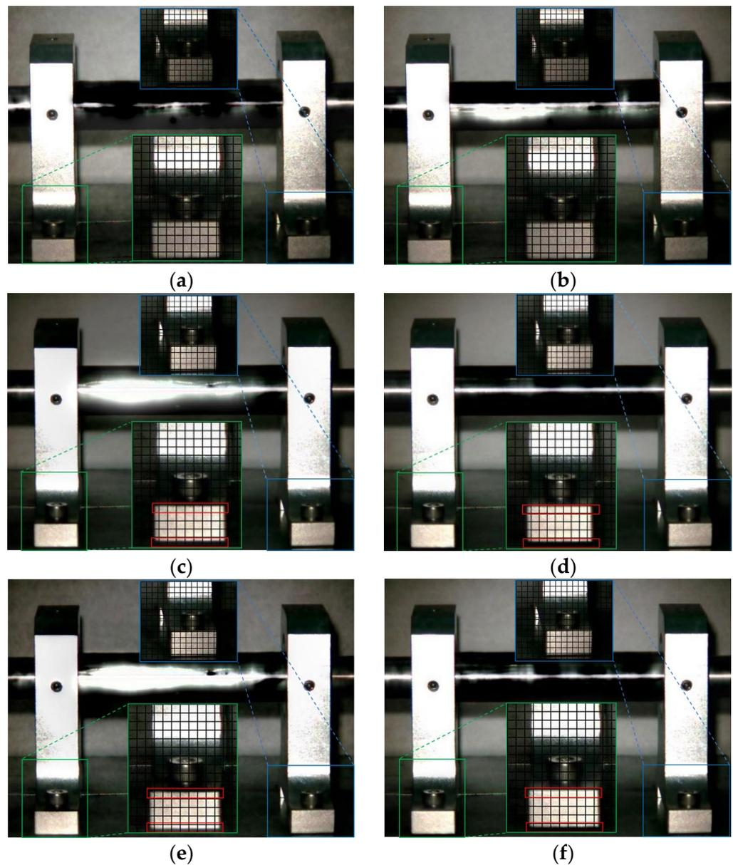
**Figure 5.** MM images of two frames at  $1\times$  frequency under condition 1 and condition 2. (a) Normal (maximum frame); (b) normal (minimum frame); (c) fault (maximum frame)—traditional method; (d) fault (minimum frame)—traditional method; (e) fault (maximum frame)—improved method; (f) fault (minimum frame)—improved method.
