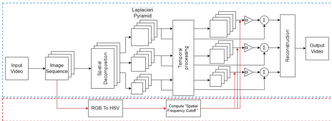
Figure 1. Improved Eulerian video motion magnification process.
