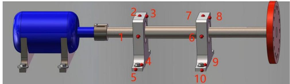
Figure 4. Diagram of vibration measurement points.
