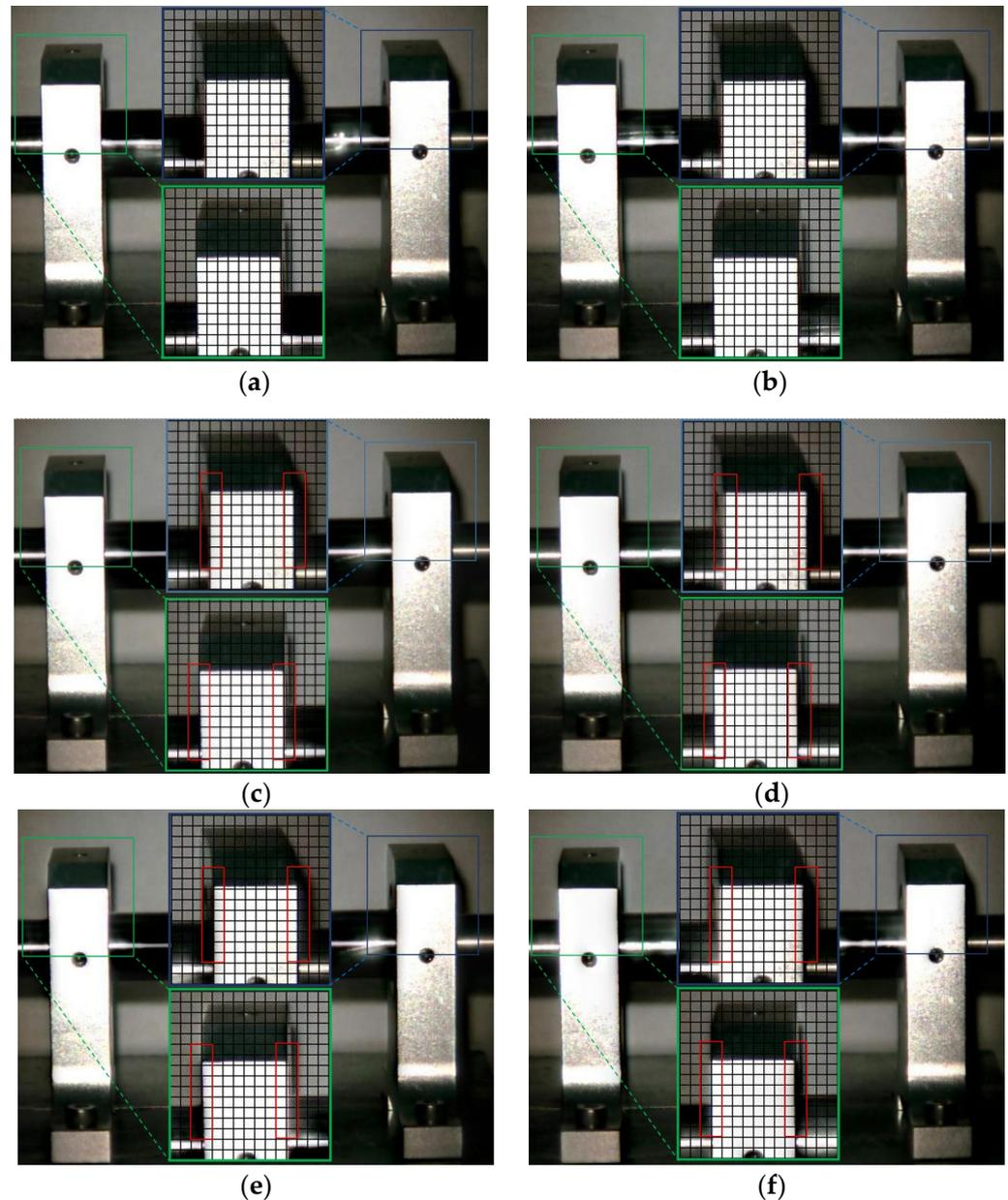
**Figure 8.** MM images of two frames at  $2\times$  frequency under condition 1 and condition 3. (a) Normal (maximum frame); (b) normal (minimum frame); (c) fault (maximum frame)—traditional method; (d) fault (minimum frame)—traditional method; (e) fault (maximum frame)—improved method; (f) fault (minimum frame)—improved method.
