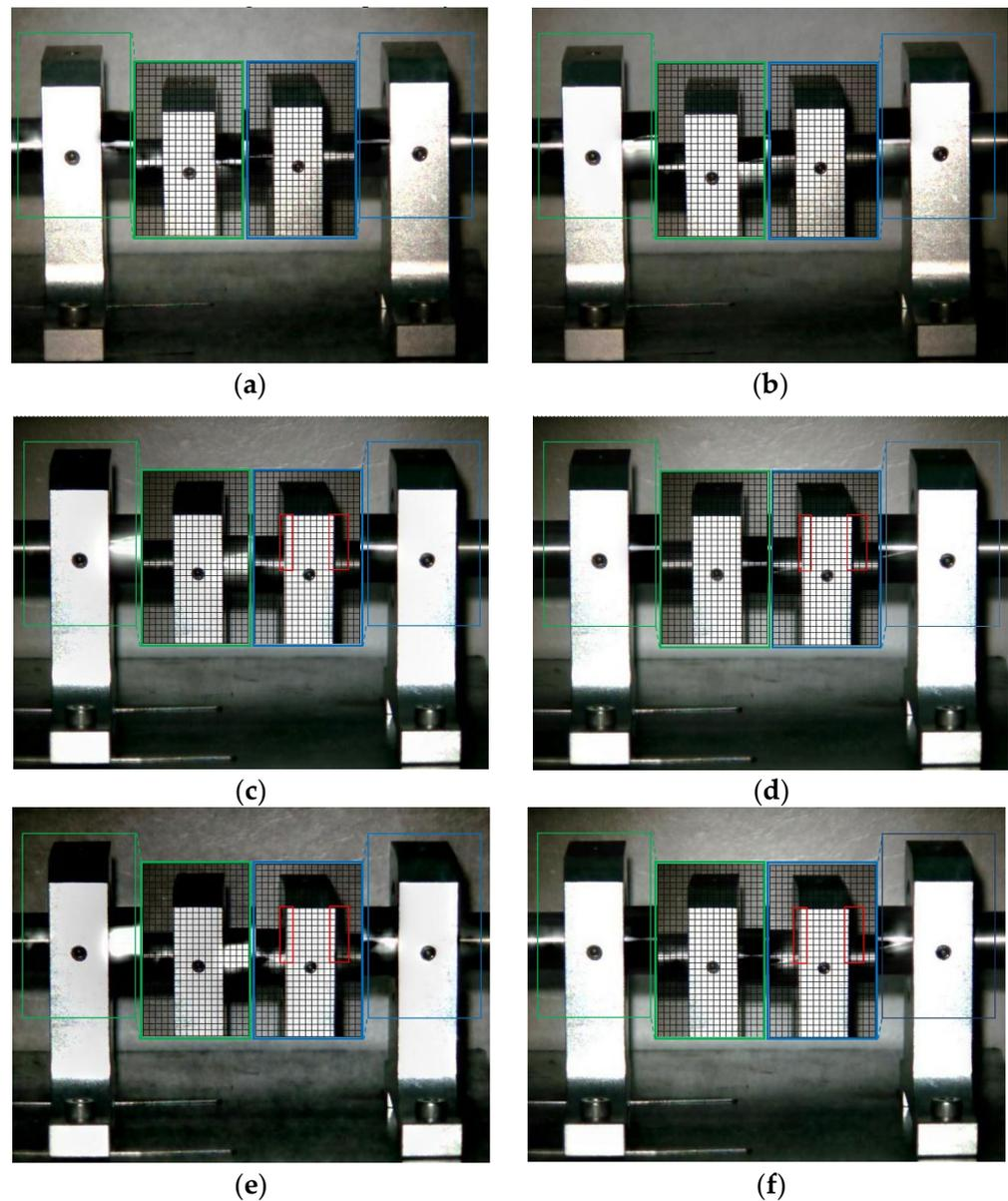
**Figure 11.** MM images of two frames at  $1\times$  frequency under condition 1 and condition 5. (a) Normal (maximum frame); (b) normal (minimum frame); (c) fault (maximum frame)—traditional method; (d) fault (minimum frame)—traditional method; (e) fault (maximum frame)—improved method; (f) fault (minimum frame)—improved method.
