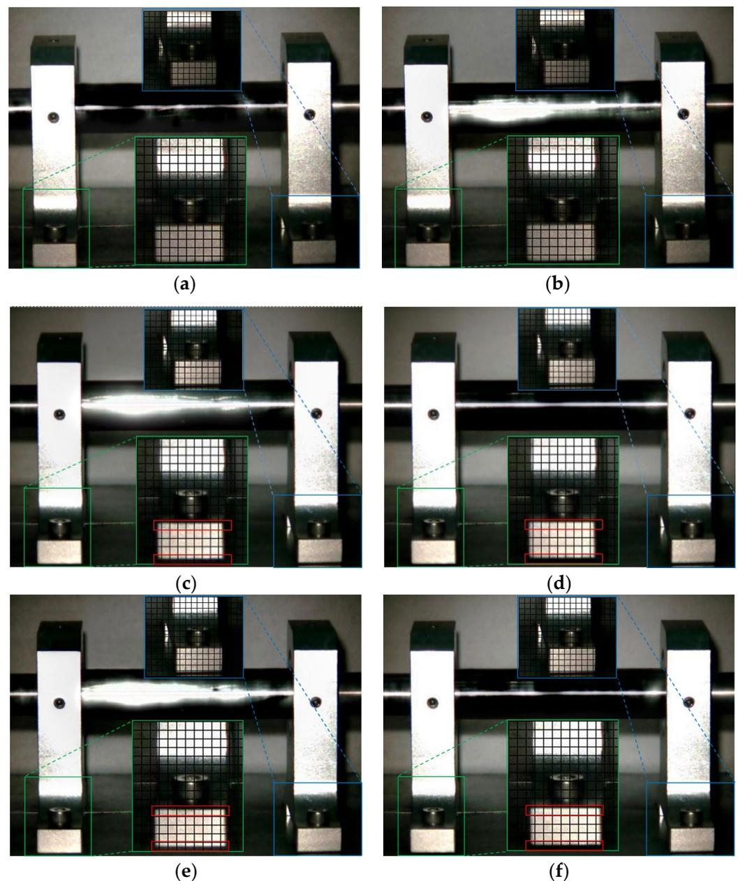
**Figure 6.** MM images of two frames at  $2\times$  frequency under condition 1 and condition 2. (a) Normal (maximum frame); (b) normal (minimum frame); (c) fault (maximum frame)—traditional method; (d) fault (minimum frame)—traditional method; (e) fault (maximum frame)—improved method; (f) fault (minimum frame)—improved method.
