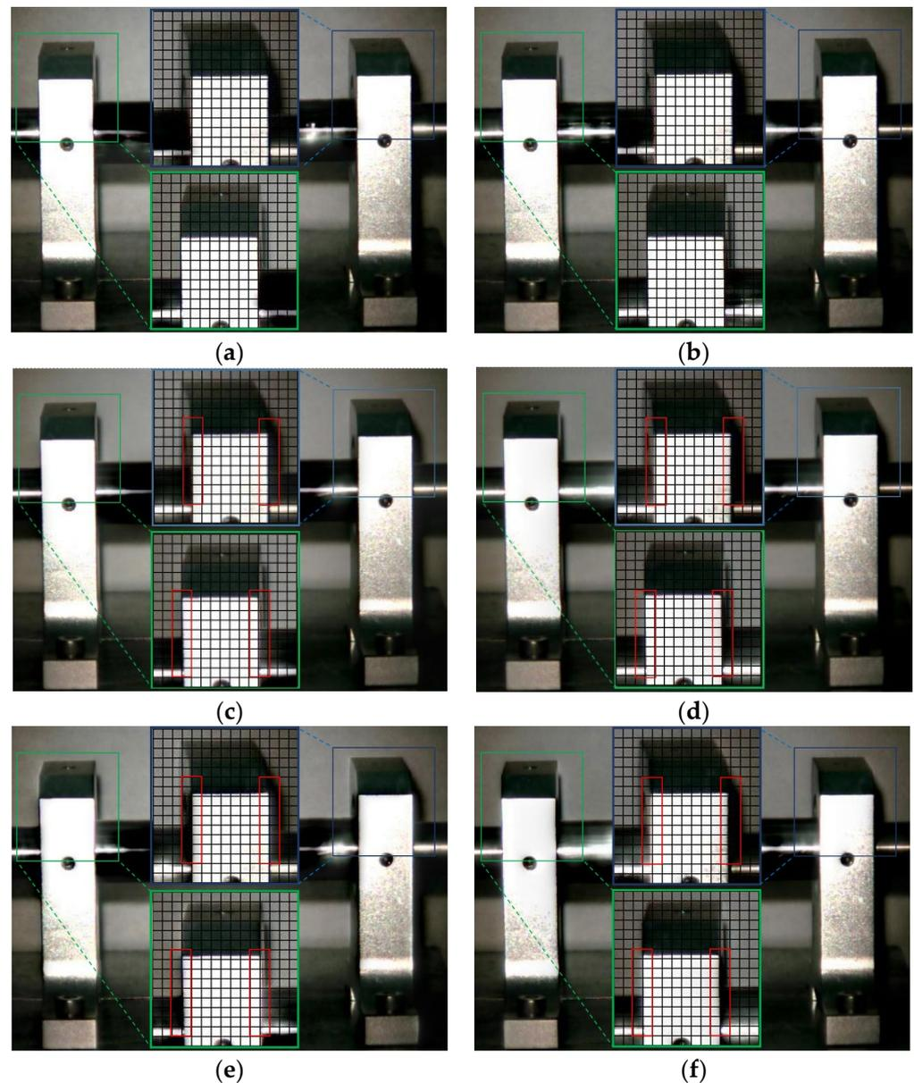
**Figure 7.** MM images of two frames at  $1 \times$  frequency under condition 1 and condition 3. (a) Normal (maximum frame); (b) normal (minimum frame); (c) fault (maximum frame)—traditional method; (d) fault (minimum frame)—traditional method; (e) fault (maximum frame)—improved method; (f) fault (minimum frame)—improved method.
