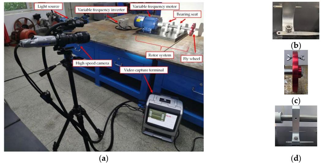
**Figure 3.** Details of the experimental setup. (a) Experimental setup; (b) condition 2; (c) condition 3; (d) condition 5.
