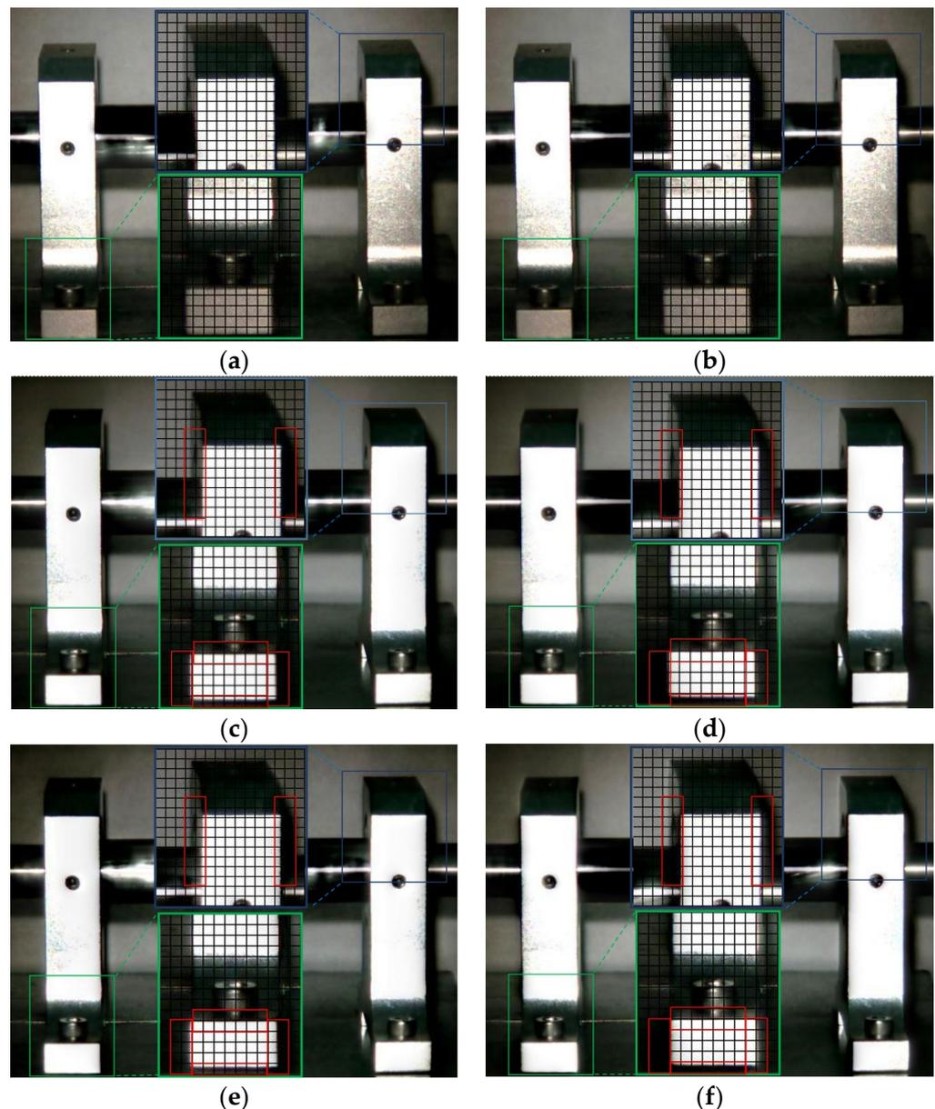
**Figure 9.** MM images of two frames at  $1\times$  frequency under condition 1 and condition 4. (a) Normal (maximum frame); (b) normal (minimum frame); (c) fault (maximum frame)—traditional method; (d) fault (minimum frame)—traditional method; (e) fault (maximum frame)—improved method; (f) fault (minimum frame)—improved method.
