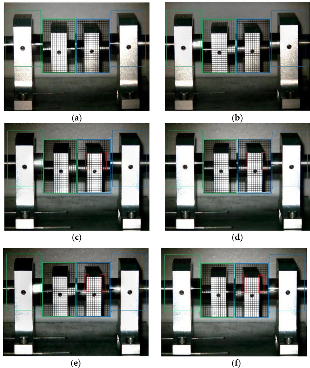
**Figure 12.** MM images of two frames at  $2\times$  frequency under condition 1 and condition 5. (a) Normal (maximum frame); (b) normal (minimum frame); (c) fault (maximum frame)—traditional method; (d) fault (minimum frame)—traditional method; (e) fault (maximum frame)—improved method; (f) fault (minimum frame)—improved method.
