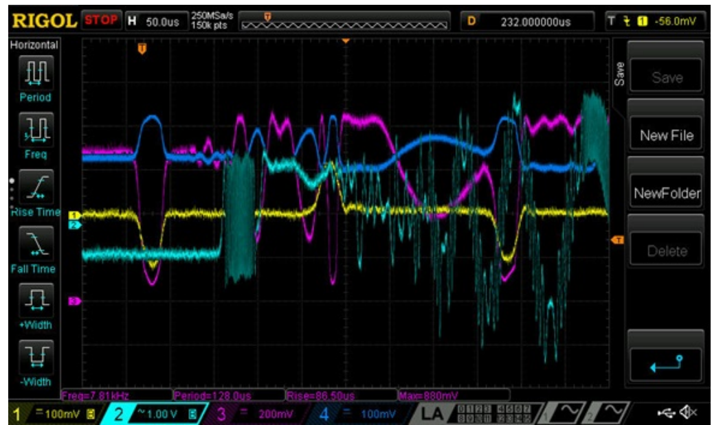
Figure 8. Screenshot from the oscilloscope screen. Waveform: 1 (yellow)—signal of the strain gauge, 2 (turquoise)—signal of the interferometer, 3 (purple)—radiation power reflected from the fiber Bragg grating, 4 (blue)—radiation power passed through the FBG. A legend is at the bottom of the screenshot. The scale on the axis 0X is 50 \mu s per division.
