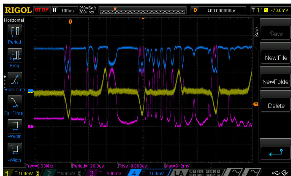
Figure 12. Waveform of signals (without the signal from the interferometer): 1 (yellow)—from the strain gauge, 2—not used, 3 (purple)—the signal caused by reflection from the FBG, 4 (blue)—the signal caused by radiation passed through FBG.
