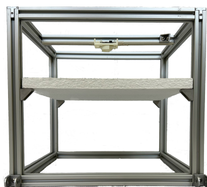
Figure 1. Experimental arrangement to fix the radar for the detection of insects.
