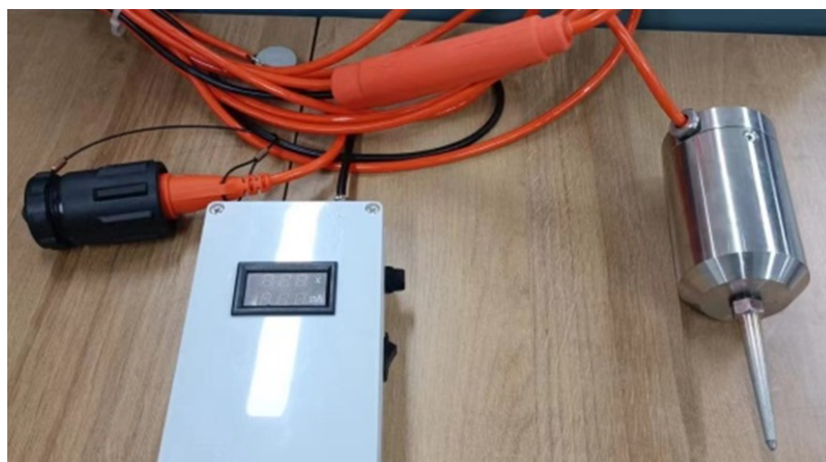
Figure 9. The prototype of the sandwiched piezoelectric accelerometer.
