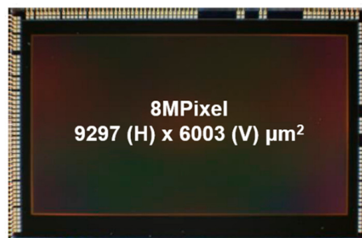
Figure 8. Chip micrograph of the 8Mp test chip.
