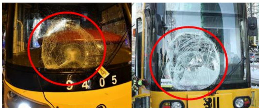
Figure 1. Windshield after collision with a pedestrian: Prague, 4 November 2019 (left) [3]; Dresden, 2 February 2019 (right) [4].
