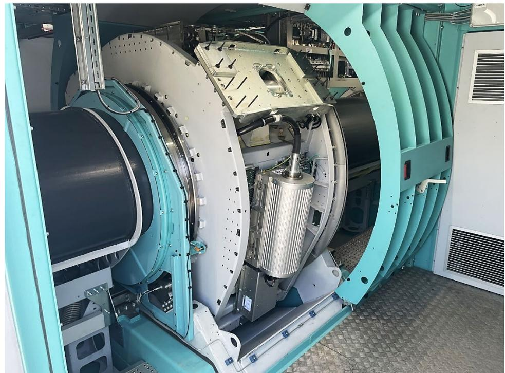
**Figure 3.** Radiation source located in the rotating portal of a CT scanner.
