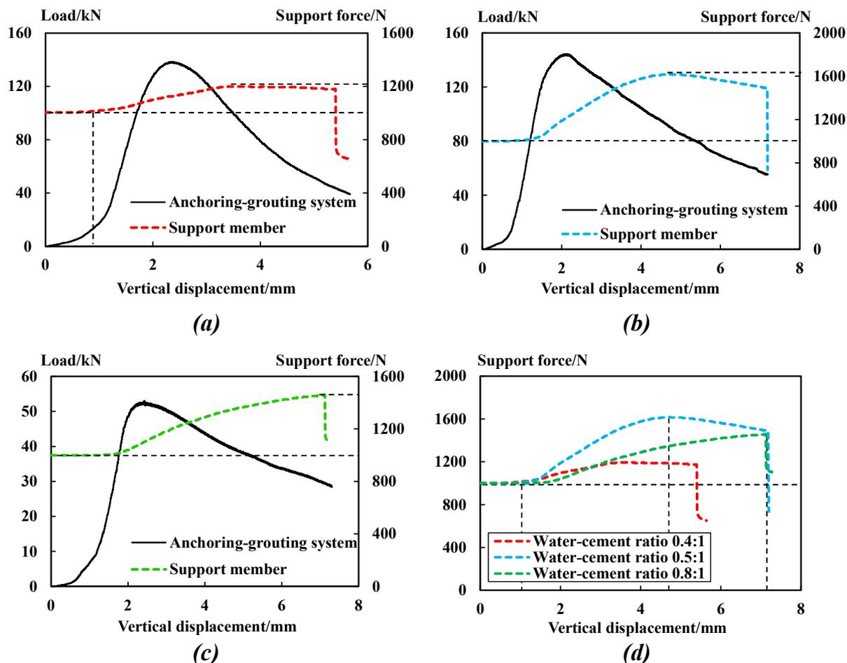
**Figure 6.** Relationship between the monitored loads/force and the vertical displacement of the anchoring–grouting system and the support members. (a) Water–cement ratio: 0.4. (b) Water–cement ratio: 0.5. (c) Water–cement ratio: 0.8. (d) Stress comparison curve of supporting members.
