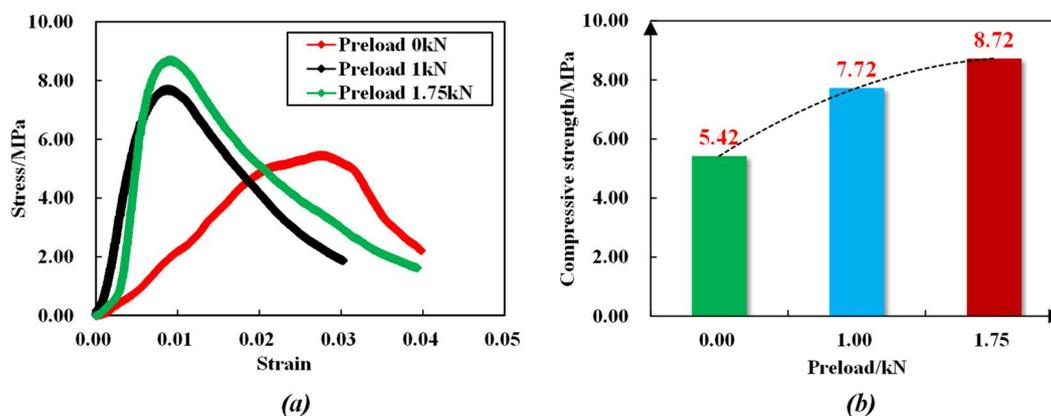
**Figure 11.** Stress–strain curve of the anchoring–grouting system with different preloads. (a) Stress–strain curve. (b) Compressive strength curve.
