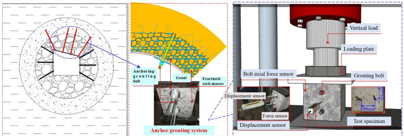
**Figure 2.** Bearing structure model and test scheme of anchoring–grouting system.
