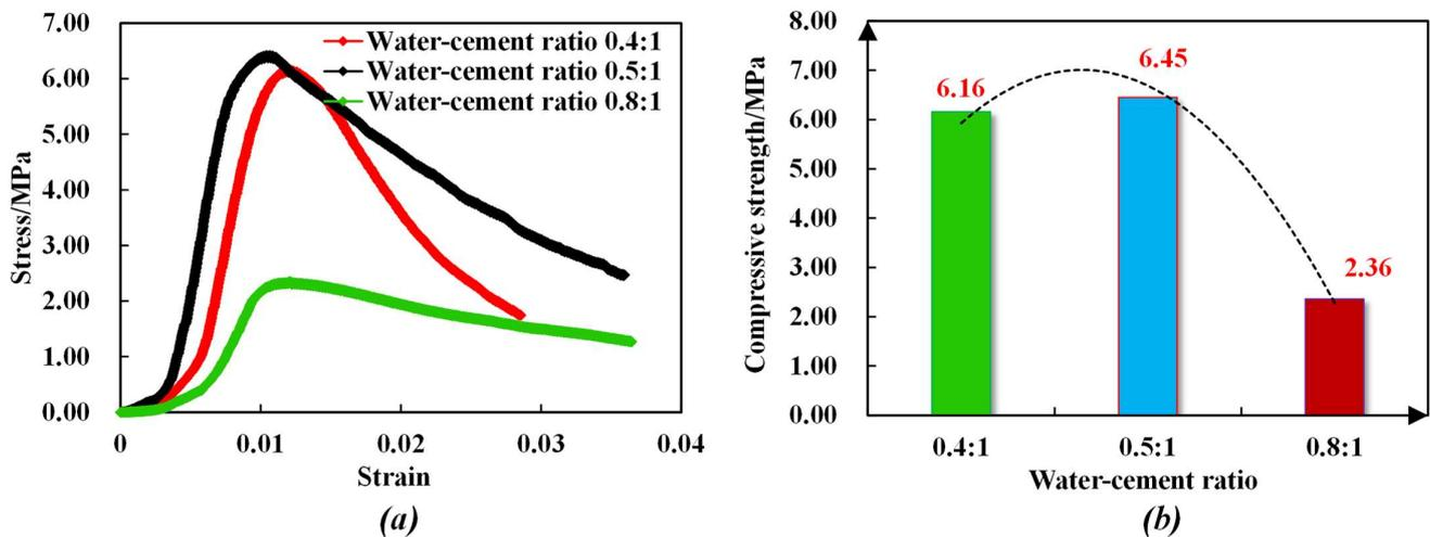
**Figure 4.** Stress–strain curve of anchoring–grouting system with different water–cement ratios. (a) Stress–strain curve. (b) Compressive strength histogram.
