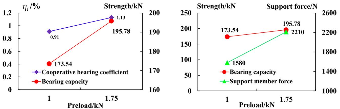
Figure 14. The cooperative bearing curve of the anchoring–grouting system with different preloads.
