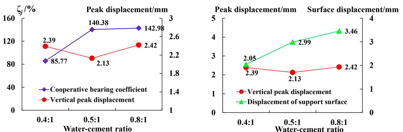
Figure 10. Coordinated deformation coefficient curve of the anchoring–grouting system with different water–cement ratios.
