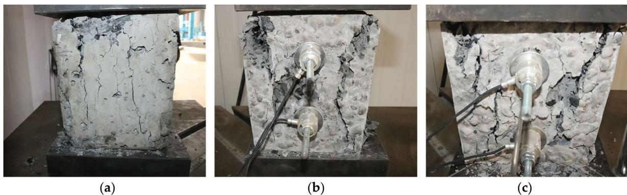
**Figure 12.** Failure modes of anchoring–grouting system with different preloads. (a) Preload: 0 kN. (b) Preload: 1 kN. (c) Preload: 1.75 kN.
