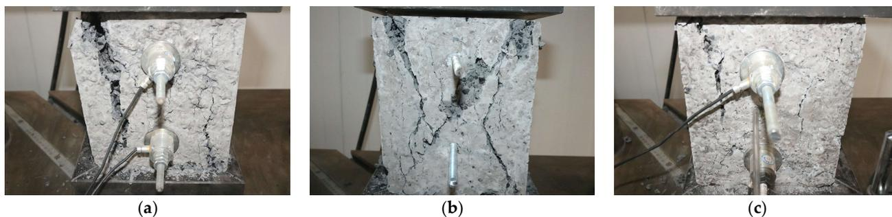
**Figure 5.** Failure modes of anchoring–grouting system with different water–cement ratios. (a) Water–cement ratio: 0.4. (b) Water–cement ratio: 0.5. (c) Water–cement ratio: 0.8.
