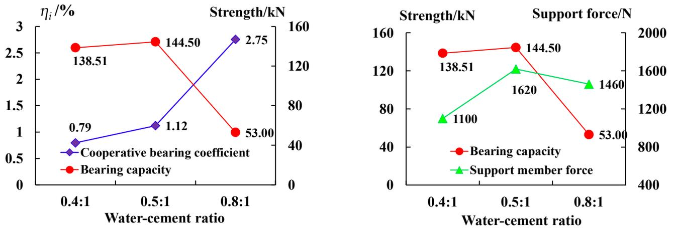
Figure 7. The cooperative bearing curve of the anchoring–grouting system with different water–cement ratios.
