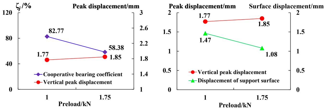
Figure 16. Coordinated deformation coefficient curve of anchoring-grouting system with different preloads.
