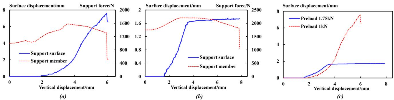
Figure 15. Displacement and force curve of supporting members. (a) Preload: 1 kN. (b) Preload: 1.75 kN. (c) Comparison curve.
