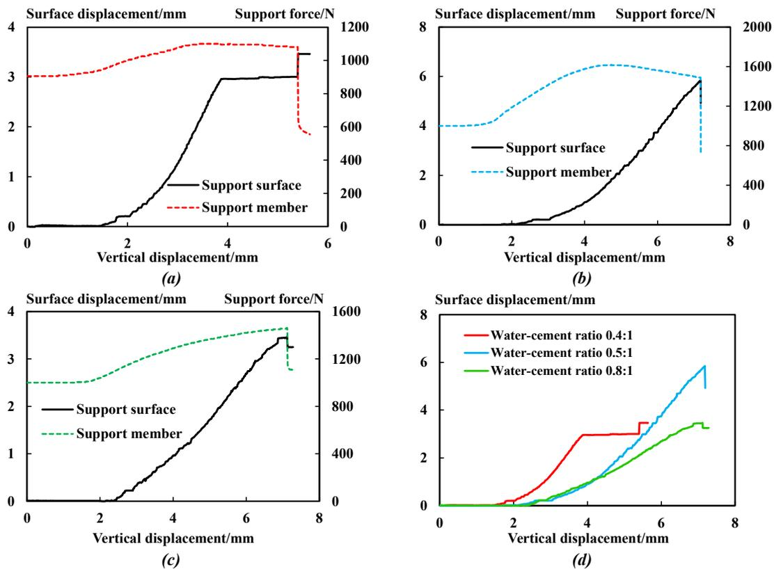
Figure 8. Stress and displacement curve of support. (a) Water–cement ratio: 0.4. (b) Water–cement ratio: 0.5. (c) Water–cement ratio: 0.8. (d) Stress comparison curve of supporting components.
