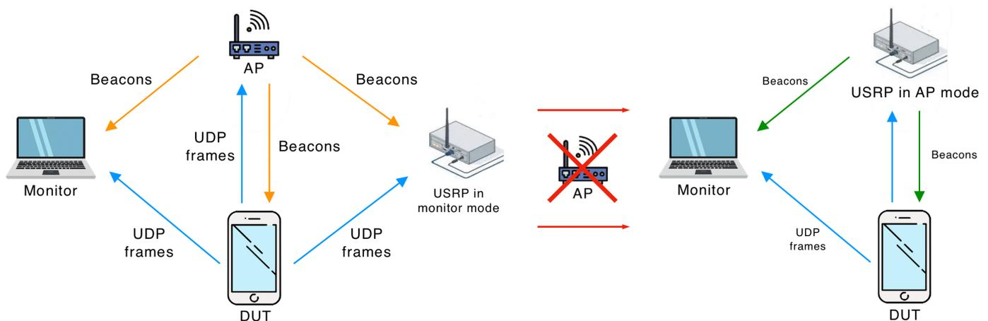
**Figure 2.** Two stages of experiment. In the first stage, the USRP listens to the AP beacons and stores them. In the second stage, the USRP sends beacons instead of the AP with added Quiet Element(s) with required parameters.
