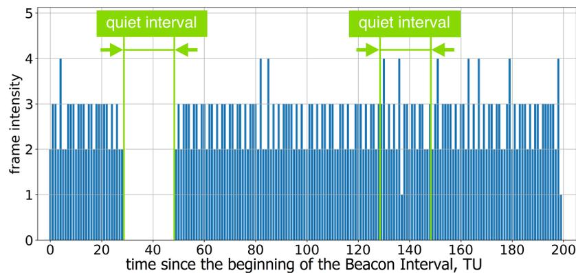
**Figure 5.** Example of frame intensity of Group A devices in Test 3 on two consecutive Beacon Intervals, each of which has an allocated Quiet Interval.
