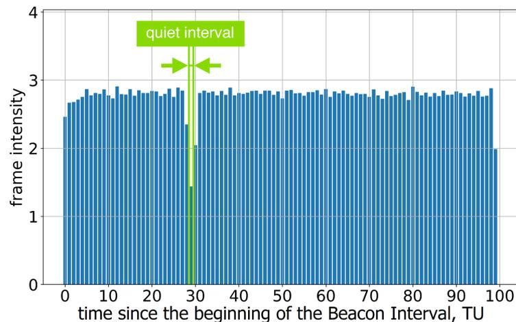
**Figure 4.** The average frame intensity of Group A devices in Test 2.
