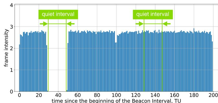
**Figure 6.** The average frame intensity of Group A devices in Test 3 on two consecutive Beacon Intervals, each of which has an allocated Quiet Interval.
