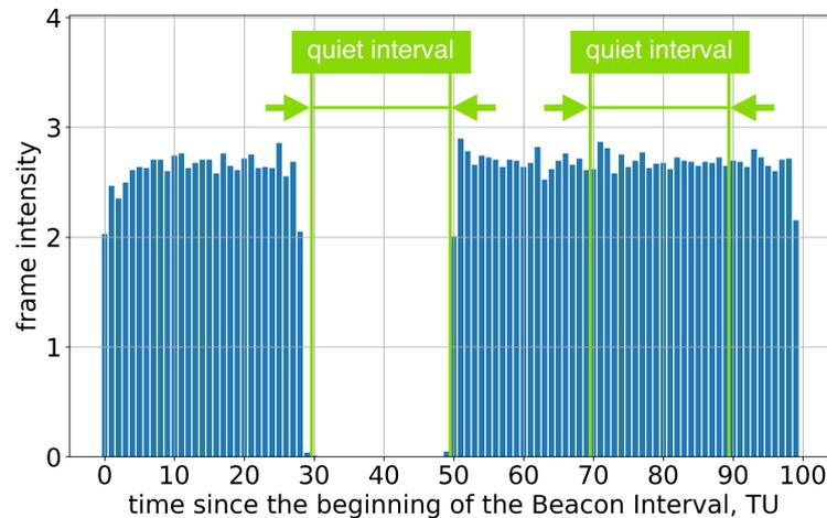
**Figure 7.** The average frame intensity of Group A devices in Test 3 with two Quiet Intervals in a Beacon Interval.
