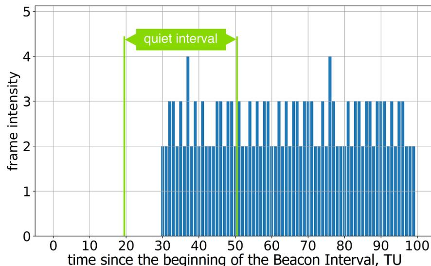
**Figure 8.** The average frame intensity of Group D devices in Test 1 with a single Quiet Interval.
