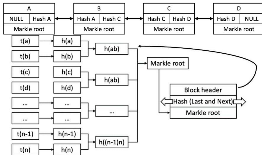
Figure 5. Blockchain communication and calculation of Merkle root.
