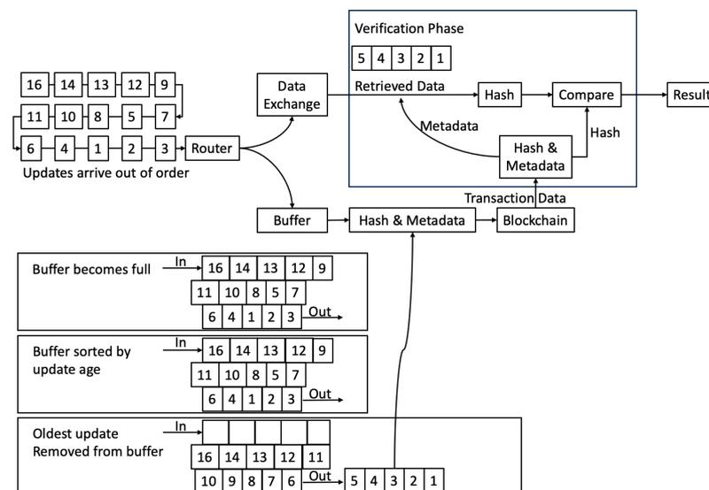
Figure 4. Blockchain communication and calculation of Merkle root.
