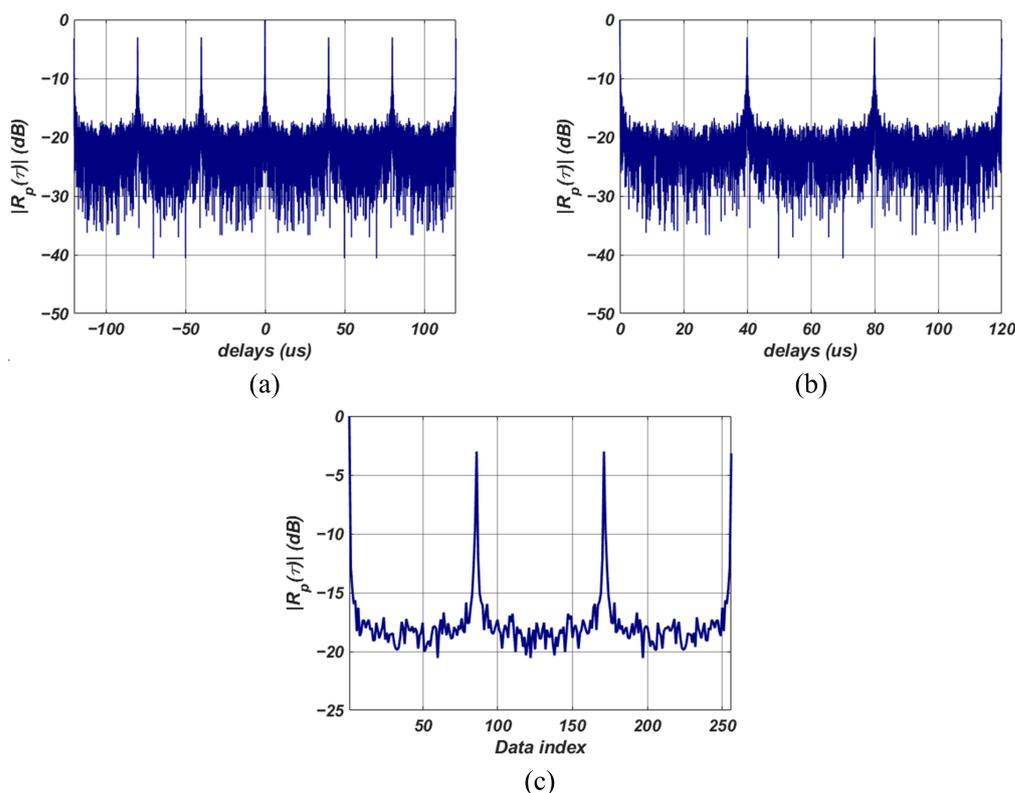
**Figure 3.** Results of the preprocessing steps. (a) decibel scale conversion process results, (b) negative delay removal process results, (c) fixed-length max pooling results.
