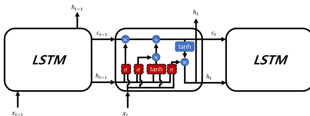
Figure 4. Architecture of the LSTM network.
