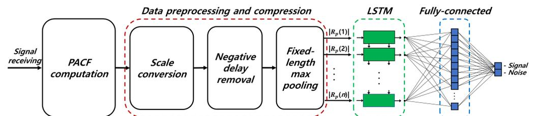
**Figure 1.** Block diagram of the proposed signal detection method.
