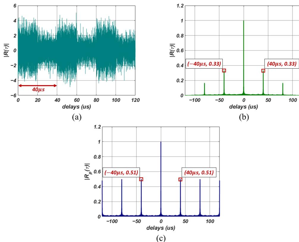
**Figure 2.** Examples of simulated radar signals and corresponding computed autocorrelation functions (ACFs). (a) Simulated LFM radar signal, (b) Computed ACF, (c) Computed PACF.
