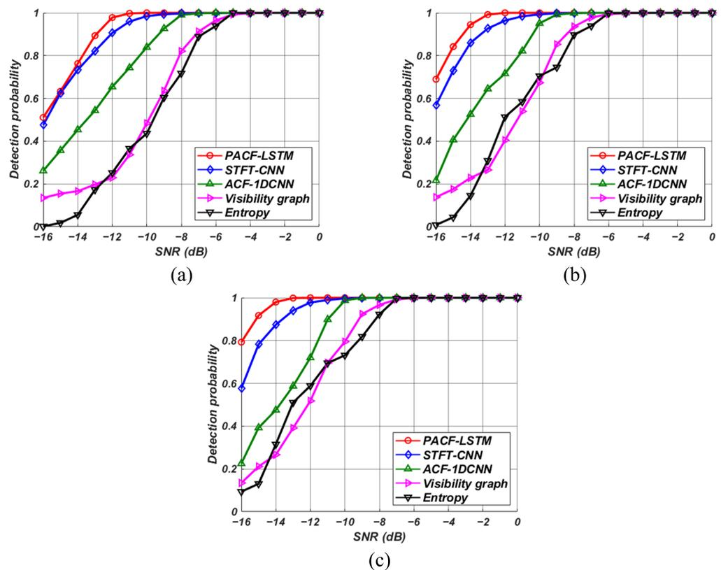
**Figure 5.** Detection probabilities of the detectors at various SNRs. Pulse width of (a) 10  $\mu$ s, (b) 20  $\mu$ s, and (c) 30  $\mu$ s.
