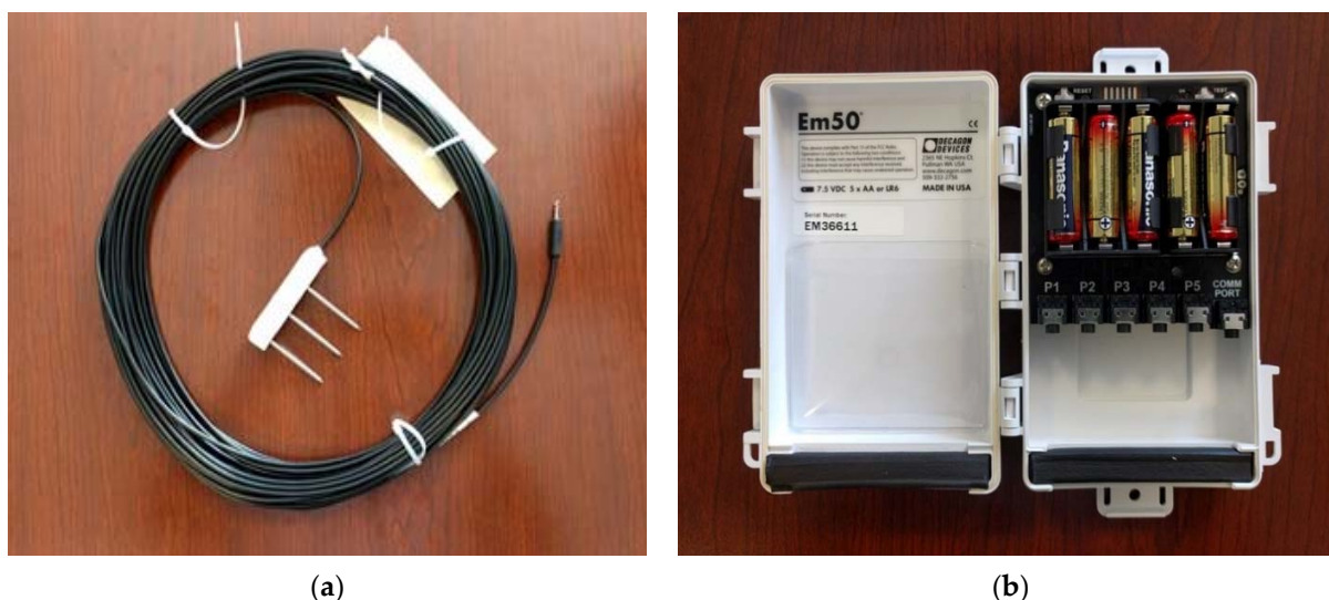
Figure 7. Sensor for measuring dielectric constant, electrical conductivity, temperature, and volumetric water content of soil. (a) Soil moisture and dielectric permittivity sensor. (b) Data logger.
