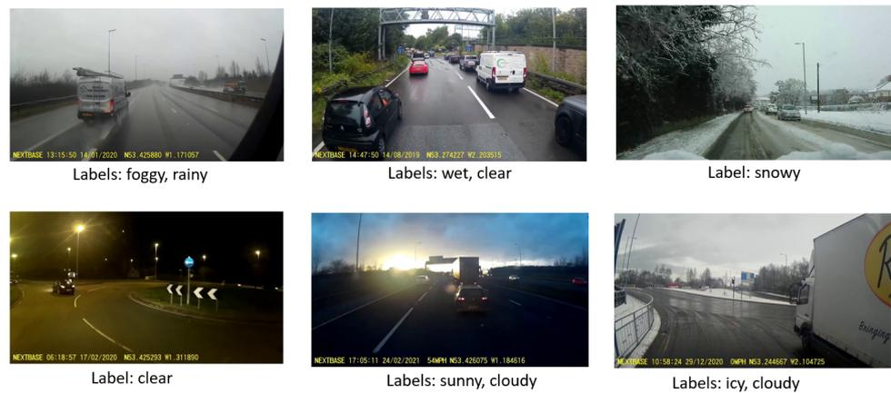
**Figure 5.** Six samples of weather images from our multi-label road weather dataset.
